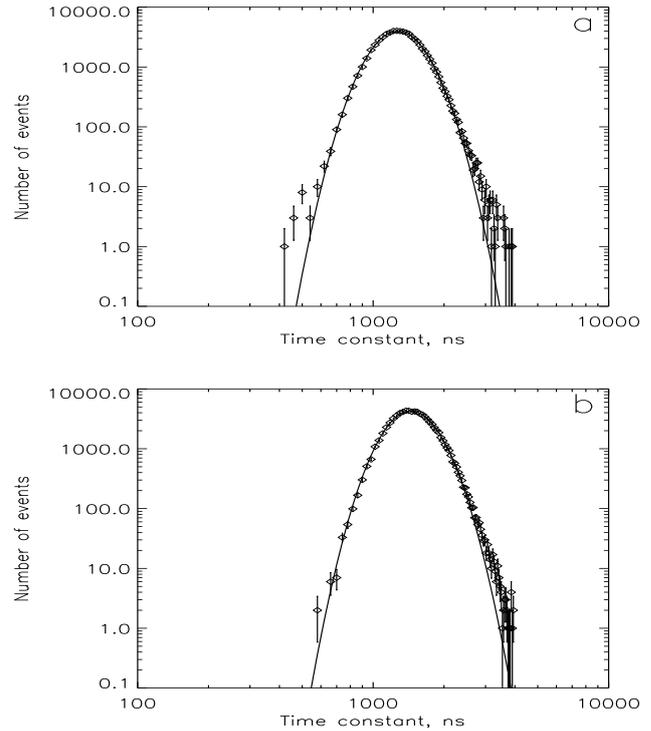
**Fig. 1.** a) Time constant distribution for events with visible energy 30-50 keV from the CsI(Tl) crystal; b) similar distribution after crystal polishing. Solid curves show fits to a log(Gauss)-function.
