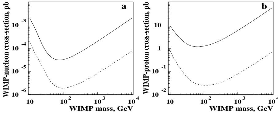
**Fig. 4.** Preliminary limits on spin-independent WIMP-nucleon (a) and spin-dependent WIMP-proton (for the case of pure higgsino) (b) cross-sections derived from the UKDMC NAIAD experiment (solid curves). Dashed curves show predicted sensitivity for 100 kg  $\times$  years exposure.
