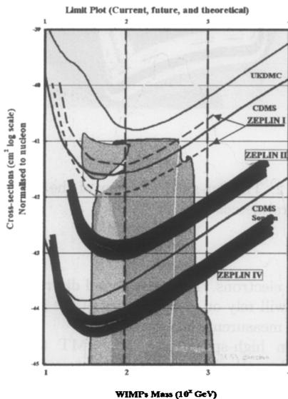
Figure 3. The expected sensitivity of the ZEPLIN-II detector.
