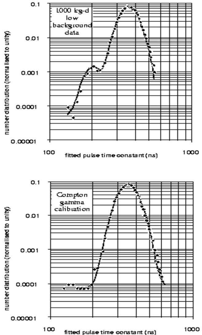
**Figure 3:** Time constant distributions (normalised to unity) for 5 kg NaI crystal: (*uppergraph*). Background distribution showing additional population of shorter pulses; (*lowergraph*). Compton calibration with  $^{60}\text{Co}$  source (5 hours each day).
