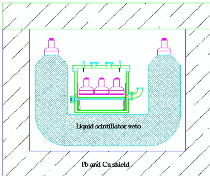
Figure 5: Two-phase ZEPLIN detector in scintillator veto
