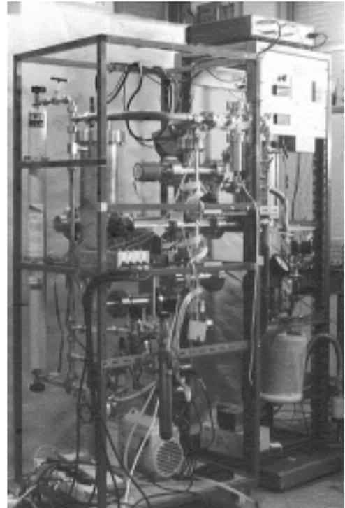
**Figure 2:** Xenon purification and liquefaction system
