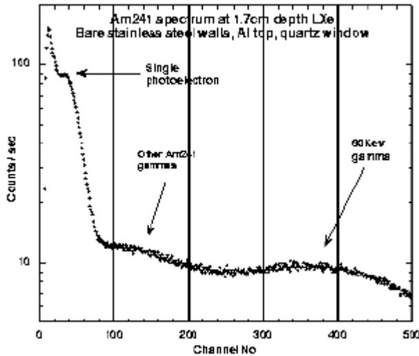
**Figure 5:** Americium gamma-ray spectrum from liquid xenon
