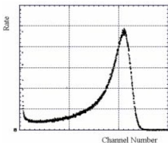
**Figure 3:** Alpha particle spectrum from 1.7 cm depth of liquid xenon
