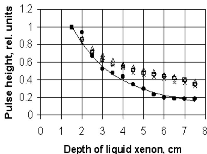
**Figure 4:** Variation of alpha peak position with depth of xenon
