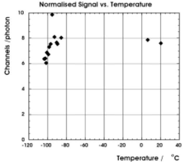
**Figure 6:** Variation of signal amplitude with temperature for an ETL 9829 PMT
