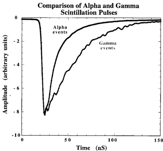
**Figure 7:** Comparative pulse shapes from alpha particle and gamma-rays
